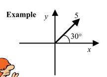
The vector of length 5 at  $30^{\circ}$  to the *x*-axis can be split into two components using trigonometry.
